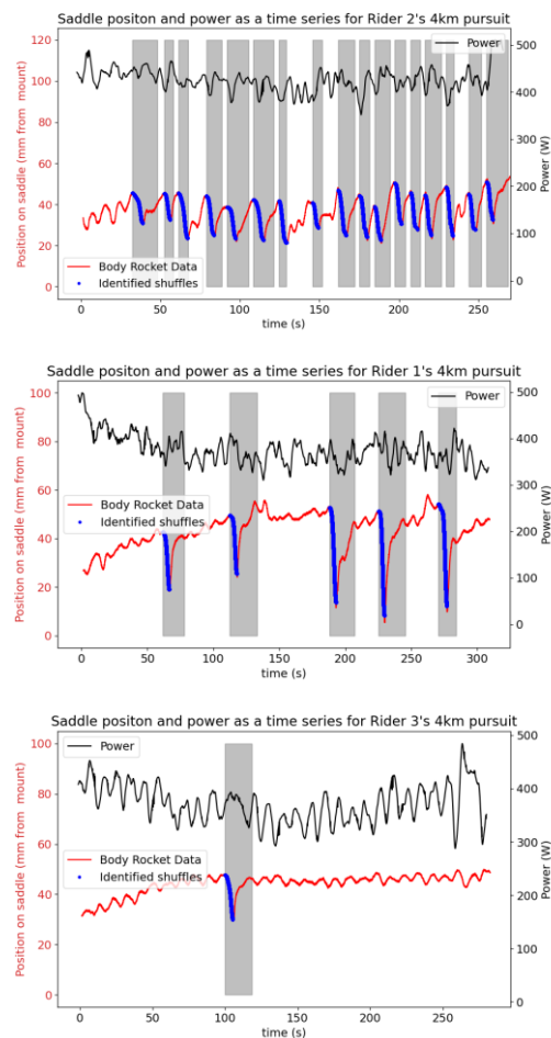
Figure 3. Rider saddle position vs cycling power output from two example riders (plots A & B) during a 4 kilometer cycling time trial. Cycling power output (black), saddle position (red) are plotted against time with identified saddle shuffles illustrated in blue with the period of the shuffle shown by the grey shading.
