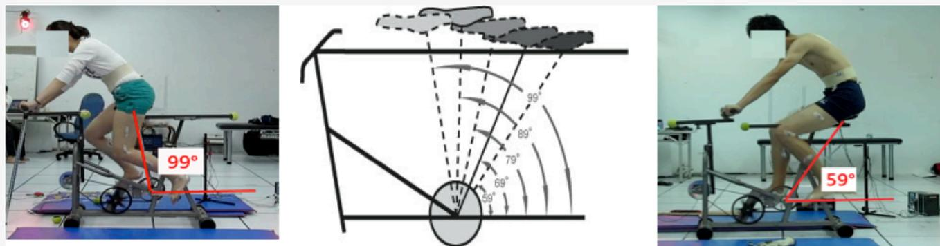
Figure 1. Five riding seat positions of different seat-tube angle conditions.
