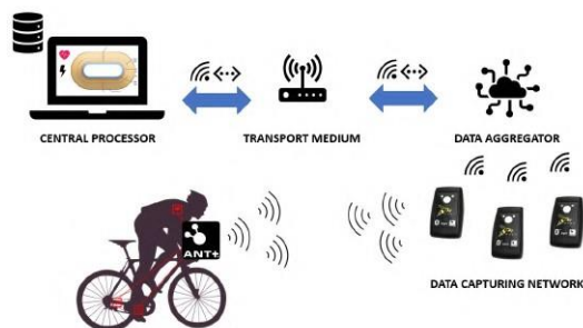
Fig. 2: Schematic overview of sensor data capturing within the WCN project.
