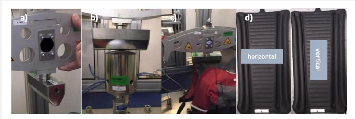
**Figure 1.** a) RIF between the FPS and the APS (20 mm thick EVA padding and 1 bar air pressure); b) RIF between different air pressure setting within the APS (with 20 mm thick padding); c) RIF between different padding thicknesses at the APS system with a constant air pressure of 1,0 Bar; d) RIF between two different alignment settings (horizontal and vertical) of the drop body during the impact on the APS with 10 mm thick EVA paddings and 1 bar air pressure
