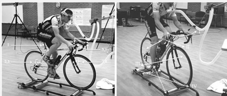
**Figure 2.** A) Reflective markers on the bicycle (seat post, seat stays, center handlebar, brake hoods, and front forks); B) Kinematic movements (steering, lean, displacement and yaw)
