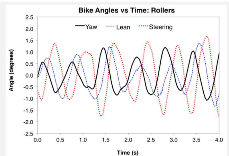
**Figure 3.** Bicycle angular motion patterns for riding on rollers for a representative rider. Yaw angle was the frame angle with respect to the forward direction in the horizontal plane. Lean angle was the frame inclination with respect to vertical in the frontal plane. Steering angle was the angle of the handlebars with respect to a mediolateral axis in the horizontal plane.
