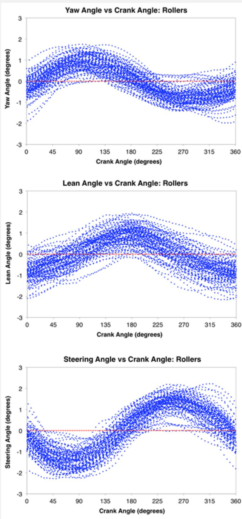
**Figure 4.** Variability of A) yaw, B) lean and C) steering angles during one minute of cycling on rollers for a representative rider. Approximately 90 crank revolutions are included in these graphs. Positive angles were left of center, negative angles were right of center. Crank angle was 0° with the right pedal at top-dead-center and 180° at bottom-dead-center.
