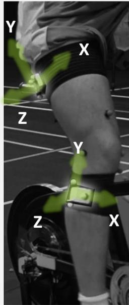
**Figure 1.** Sensor positioning on thigh and shank local axis
