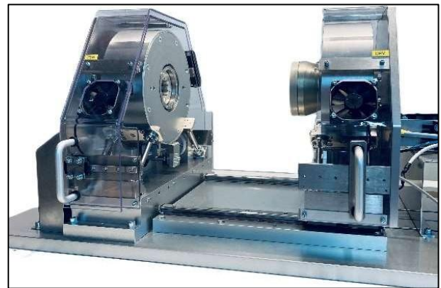
Figure 1. Hub-level efficiency testing
